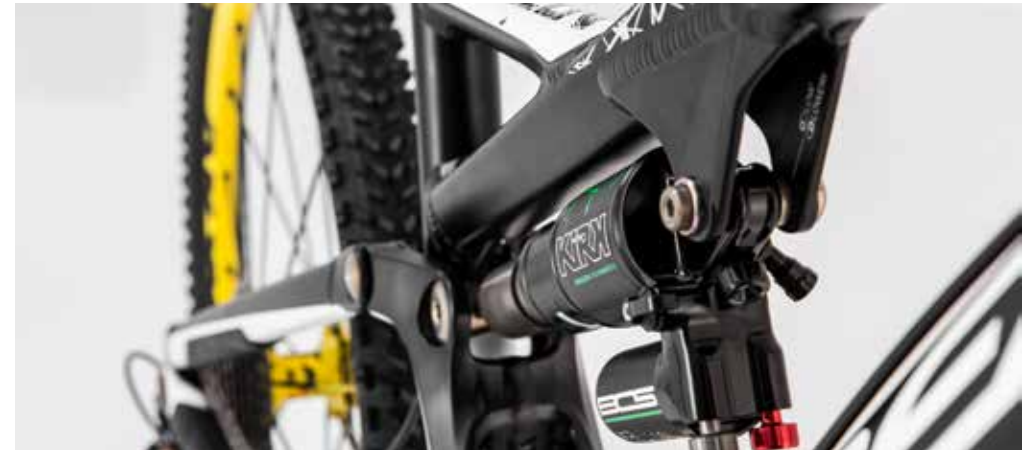
PRESSURE AND REBOUND CLICKS: The values provided in the chart are just a starting point, in order to achieve maximum performance the shock setup should be suited to the rider and terrain. COMPRESSION ADJUSTMENT FOR KIRK SHOCK: 12 clicks counted from completely open is the recommended starting point both for low speed and high speed compression damping.
